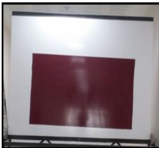
Figure 10 Scanning of the test area covered with dark red foil.
