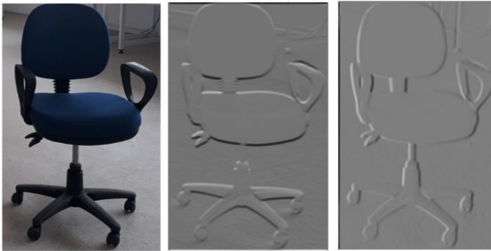
Figure 7: Gradient operator application using vertical and horizontal masks
