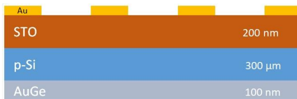
Fig. 1: Schematic representation of Au/STO/p-Si/AuGe structure
