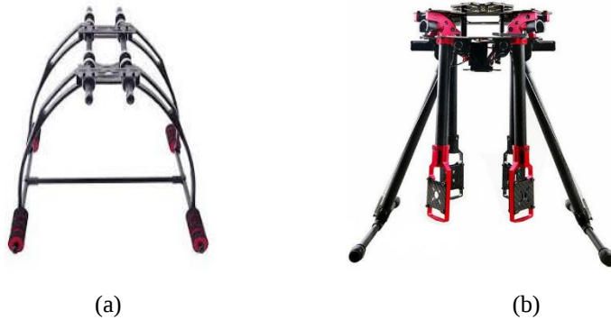
Figure 4. Examples of (a) fixed and (b) movable landing gear (İzgöl, 2021).
